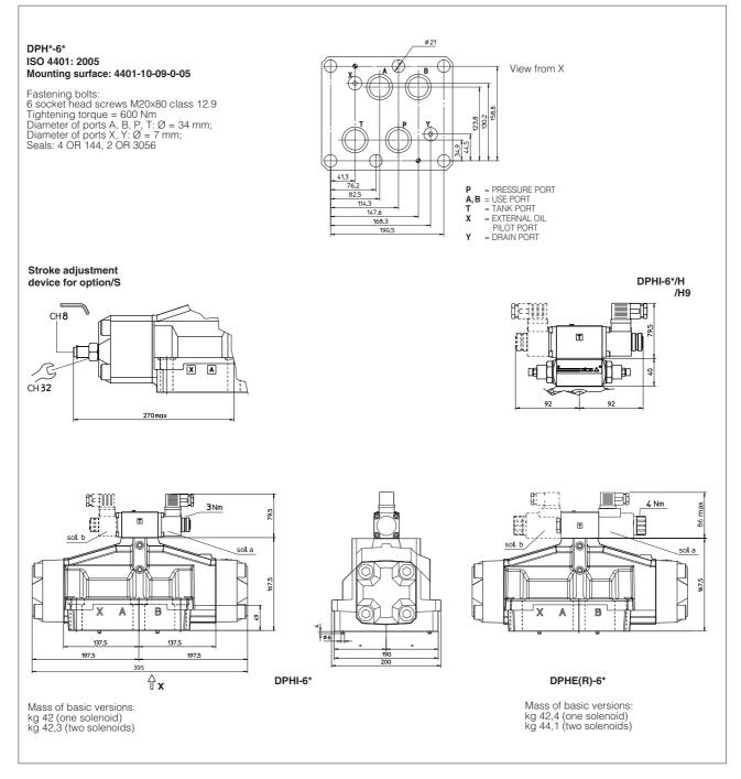
Overall dimensions refer to valves with connectors type 666
