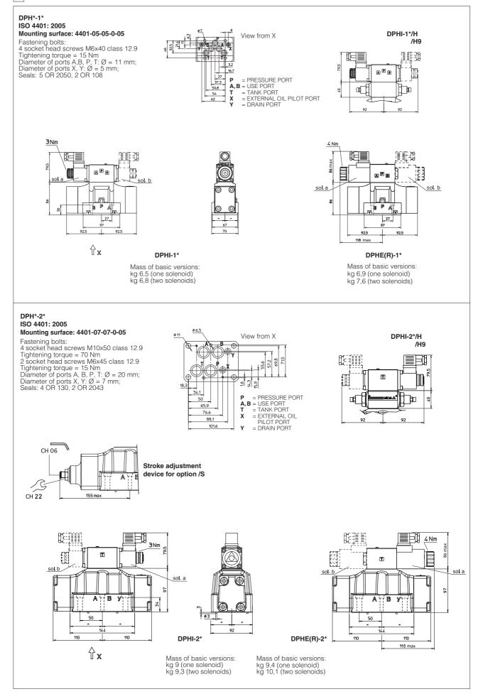
Overall dimensions refer to valves with connectors type 666
